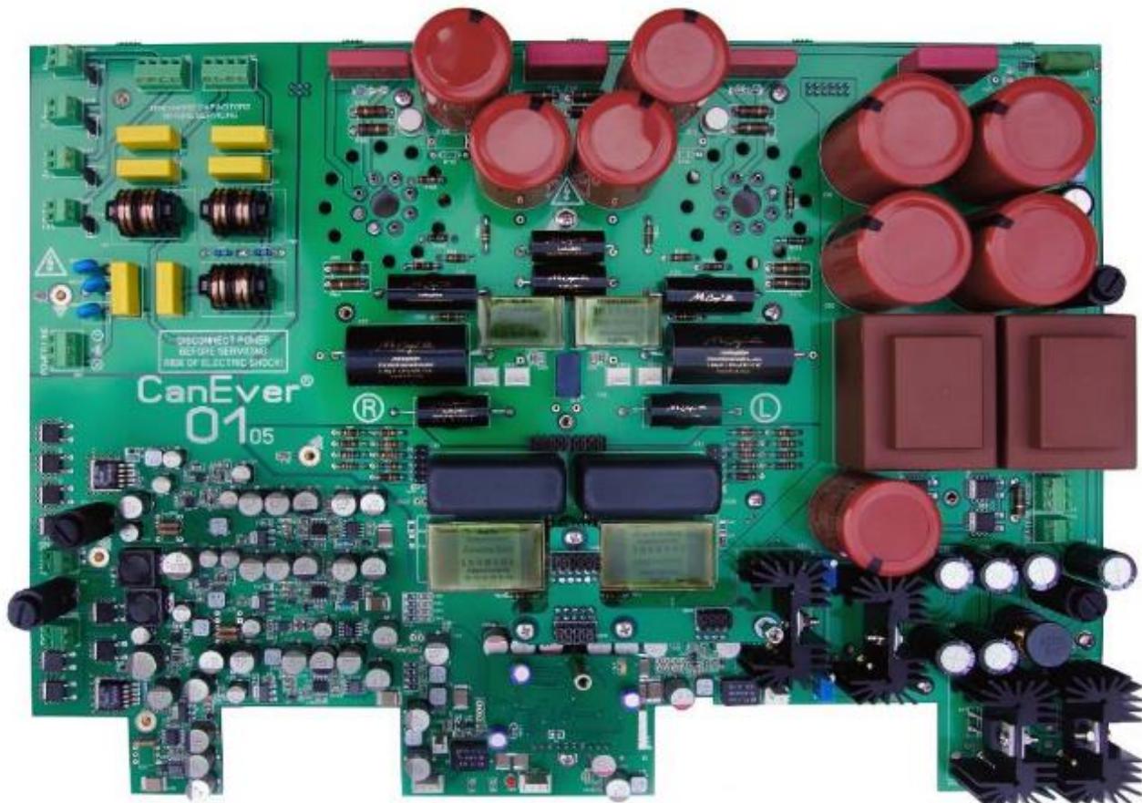
Fig. 3: The board with the Tube output stage, its power supplies, the DAC unit and the mains filters
