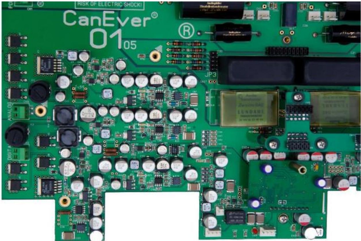
Fig. 10: The DAC circuit and the USB bridge board; SABRE 32 chip behind the USB bridge board.
